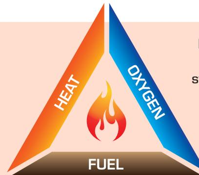
Fogmaker's fire suppression system handles all three sides of the fire triangle: heat, oxygen, and fuel. The system deploys when the protected area becomes too hot, and sprays a water-based mist that expands and chokes the fire. The mist also cools the area for a long time - at least double compared to other certified systems\* - which prevents reignition.
