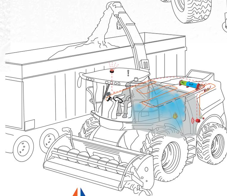
The system is tailored for different types of Agricultural machines. It is important to us to make a risk analysis with the customer prior to installation.
